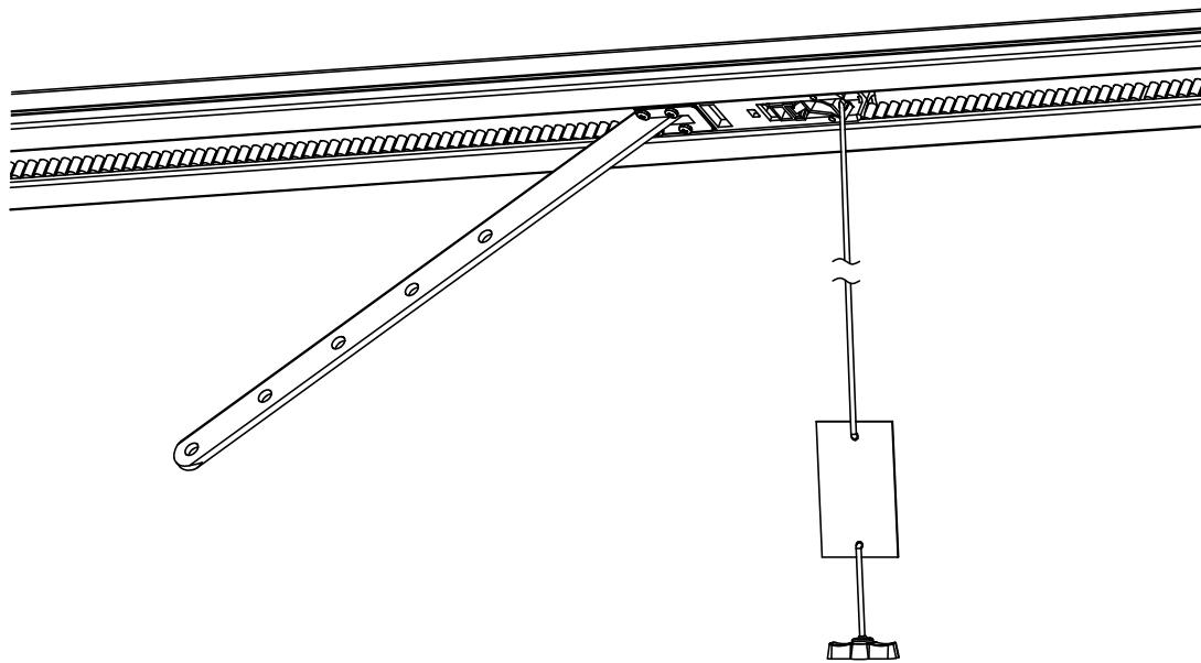
The opener is equipped with a manual release cord to disengage shuttle and move door by hand while holding the handle down. Pull on the handle to disengage the shuttle. To re-engage the door simply run opener in automatic mode or move door by hand until the trolley engages in the chain shuttle.
