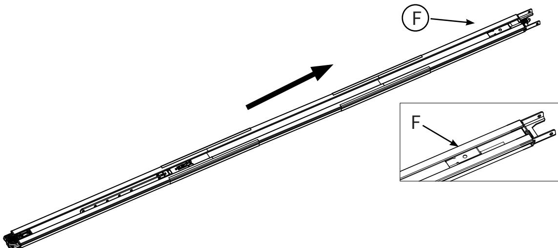
Cut the plastic thread; pull the screw rod along with inner chain to the end rail position.
