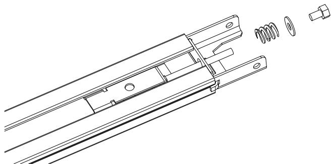
④ Tight the nut to the right position as shown, cut the plastic tape, cut the plastic thread on sprocket, then whole rail assembled finished.
