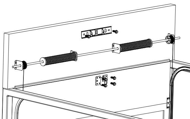
**Wall Bracket** - Close the garage door and measure the garage door width at the top and mark the centre. Locate and mount the wall bracket 2cm-15cm above the door on the inside wall. (Depend on the actual installation space).
