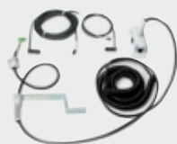
Optical edge sensors kit, TX 6m cable, RX 1m cable, electronic box, spiral cable coil cord with 3.5m or 5.5 m active length for 5.0m high door
