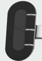
Sun visor transmitter SVR 02, 868MHz, 2 buttons, 2 channels, rolling code technology, 80m control range
