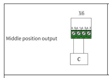
3. The external relay (C) of the dock leveler is connected to the terminal X6-6.0/6.3 of the door control device.
