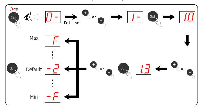
Function description: This function fine-tunes the lower limit of motor.
