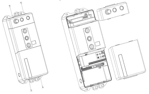
2.Connecting the Control Box Cable/Control Box Power Cable
