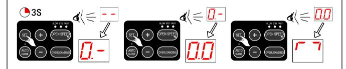
2.Check motor output direction and door direction
